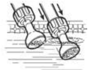
Double function nozzle: specially designed for debris at the bottom and corners.
